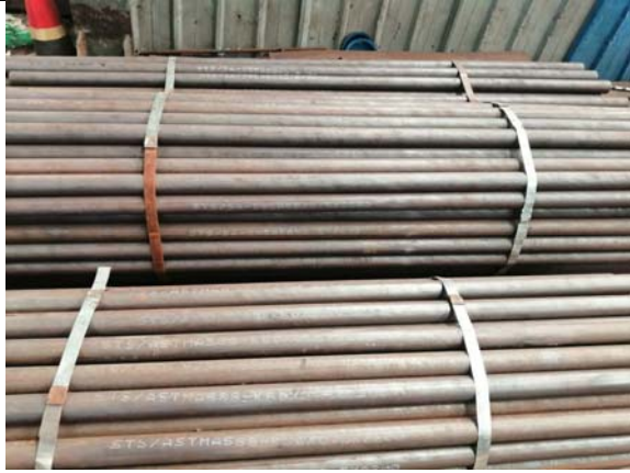
Visual inspection ( Outer surface is slightly rusted)
