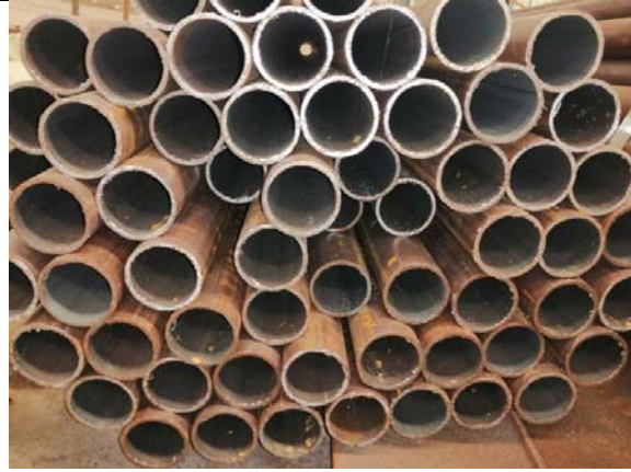
Visual inspection (Outer surface is slightly rusted)
