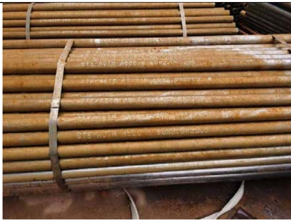
Visual inspection (rusted on the outside and inside surface)
